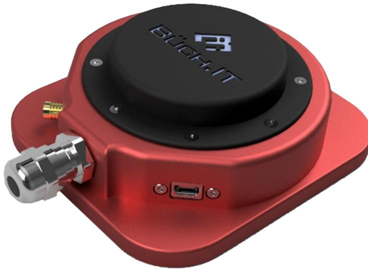
The gps100.ADAS is an All-in-One Solution to measure velocity, position and movement of a vehicle. The system is weatherproof and designed to mount on top of a vehicle.
